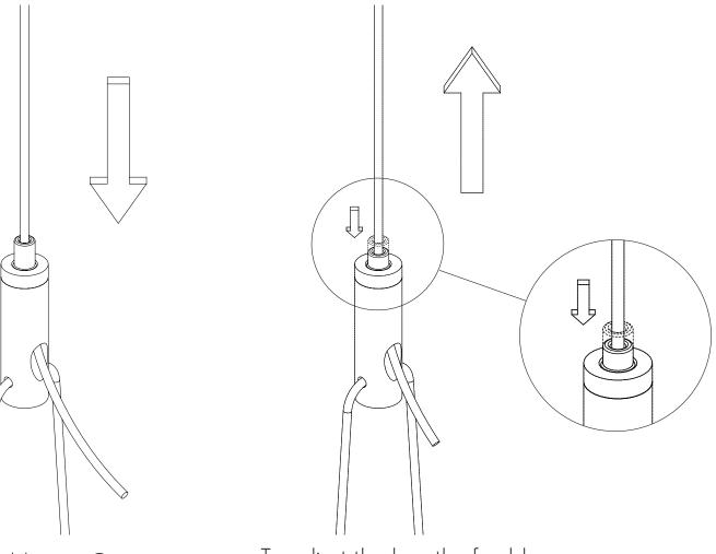
Feed AC Cable into Gripper
