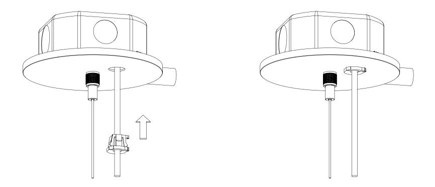
Snap the strain relief onto the wire and insert the assembly into the canopy thru hole.
