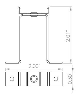
Elevate your Scout Fixture above your driver for simple wiring and installation`
