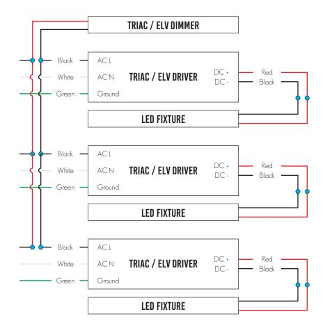
Multiple fixture wiring to single phase Dimmer
