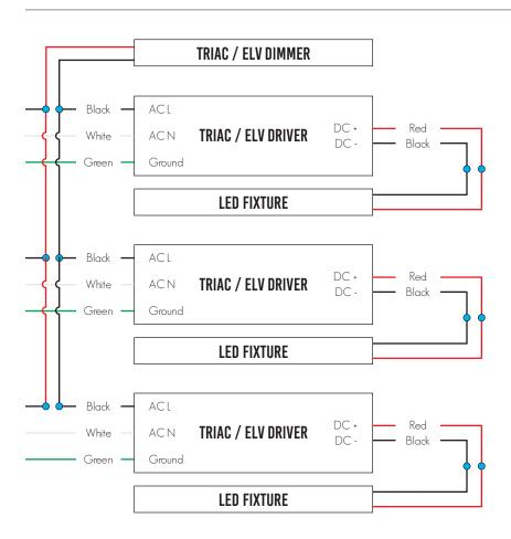
Multiple fixture wiring to single phase Dimmer
