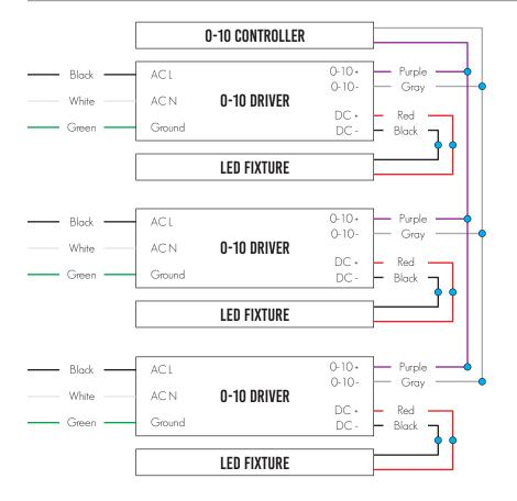
Multiple fixture wiring to single 0-10 Dimmer
