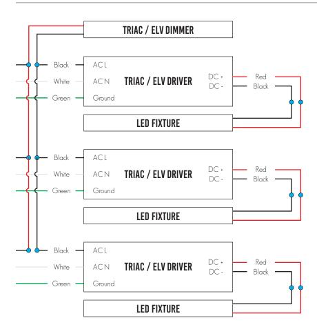
Multiple fixture wiring to single phase Dimmer
