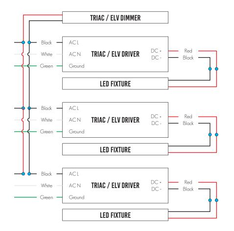
Multiple fixture wiring to single phase Dimmer
