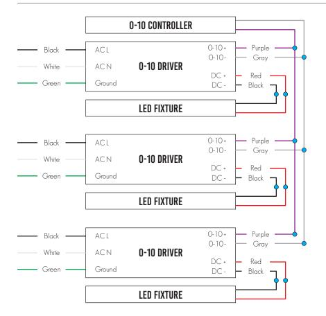
Multiple fixture wiring to single 0-10 Dimmer
